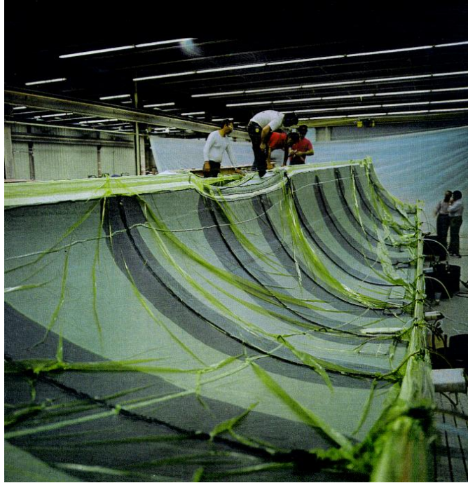
Figure 92 SCRIMP process to make a 64-foot boat
