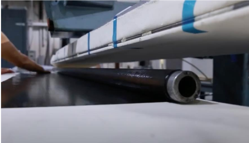
Figure 85 Roll wrapping operation
