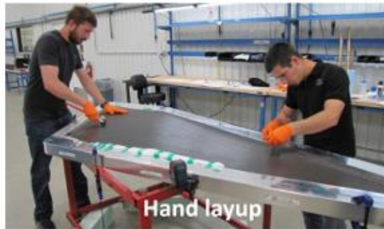
Figure 78 Hand layup of prepreg
