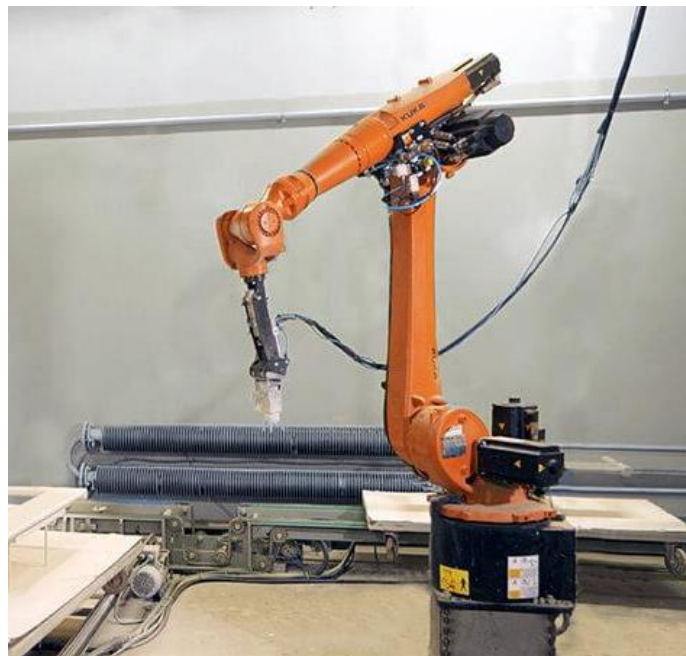
Figure 103 Ultrasonic testing using a robot and water spray
