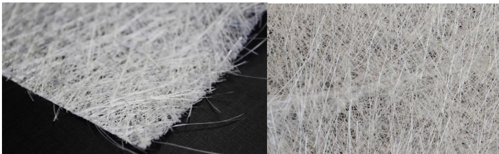
Figure 35 Chopped strand mat (left) and continuous strand mat (right)
