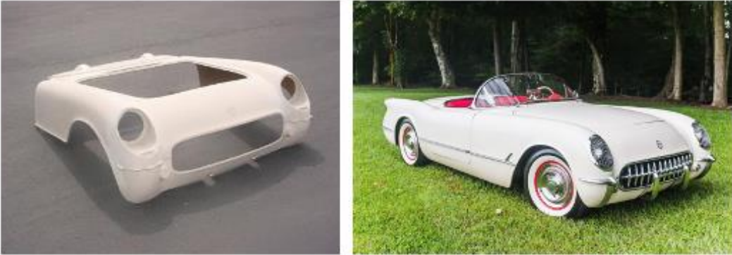
Figure 88 Corvette body made with SMC
