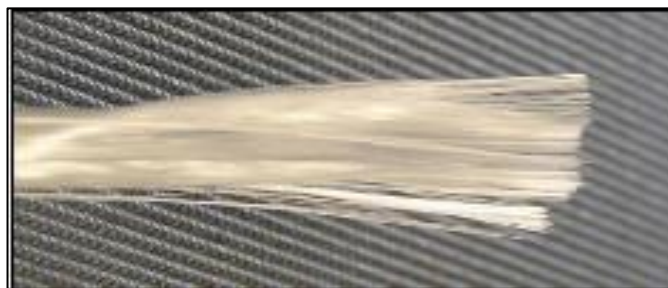
Figure 25 A fiberglass bundle (roving) that is separated to show the fibers
