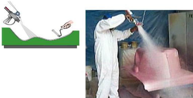
Figure 76 Sprayup method for making fiberglass composites
